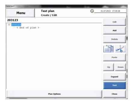
The test steps will be added in the order they will be used later. Every new and pasted test step will be added after the selected test step. The test plan will be executed top down.
