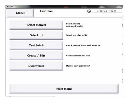
Using the button **Select** manual a new window will be opened where you can choose and start previously created test plans.
