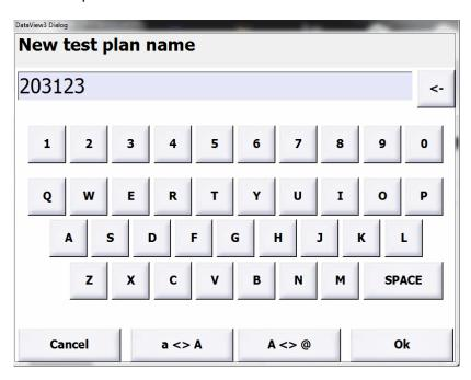
Type in the name of the test plan. As the name of the test plan is the name of the file too, you cannot use characters that Windows does not allow for file names. Close the window by pressing Ok.
