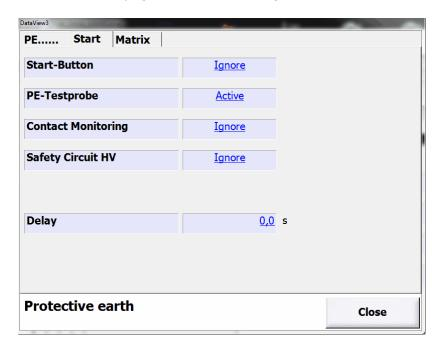
Configure the settings so that the status of **PE-Testprobe** is **Active** and of all others **Ignore**. Set the time in **Delay** to 0.0.
